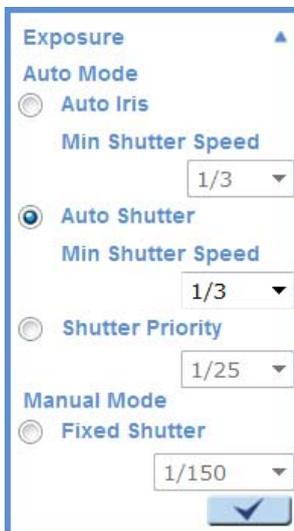
The exposure is the amount of light received by the image sensor and is determined by the width of lens diaphragm opening, the amount of exposure by the sensor (shutter speed) and other exposure parameters. With this item, users can define how the Auto Exposure function works.
