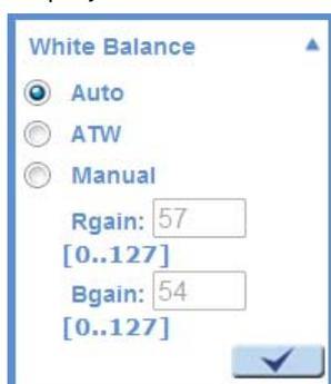
To display natural colours, the camera needs to know the reference colour temperature of the light source. Based on this reference colour temperature the camera will calculate the correct values for all colours. The camera can perform a measurement by itself or the user can set up the reference colour temperature manually. The scale unit of the colour temperature is Kelvin [K]. The following list shows the colour temperature of some light sources for reference.
