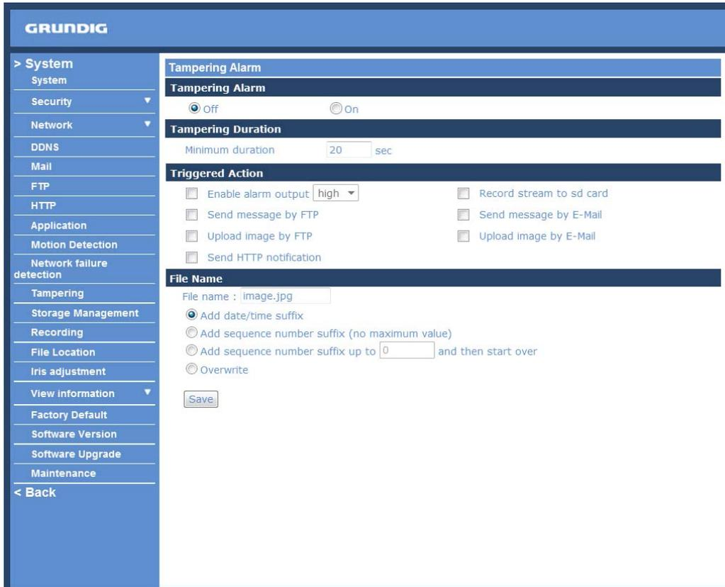
Detection of camera tampering is achieved by measuring the differences between the older frames of video (which are stored in buffers) and more recent frames.
