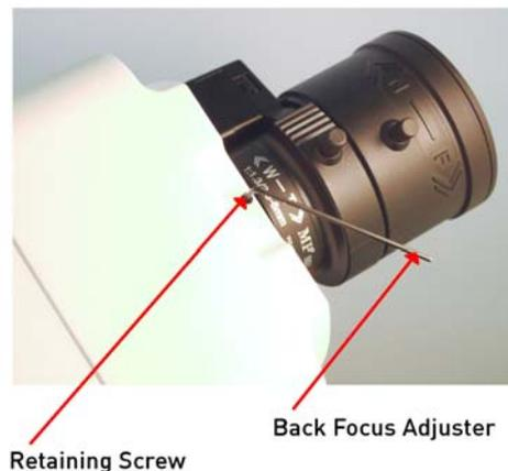
Step 2: Make sure the iris is wide open. Therefore, it is advised to keep the environment in low light condition. To open the automatic lens completely, please use a neutral density filter. With this filter it is possible to simulate a low light condition so that the lens can open up completely.
